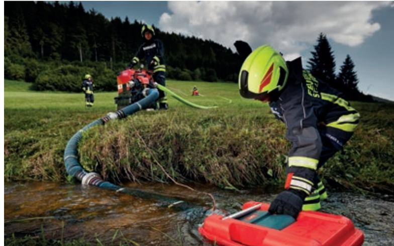
Both portable pumps can be refueled during operation. This is approved and certified by TÜV.
