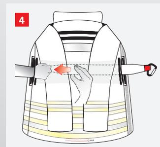
The belt is fully inserted and the two loops that can be attached to a carabiner.
